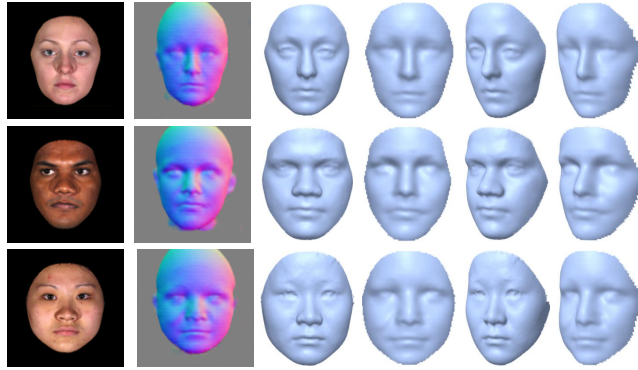
Figure 9: Reconstruction results for three BU-3DFE examples from two different viewpoints. From left to right: input image, normal map ( N ), front-view ground-truth model, front-view reconstructed model, slide-view ground-truth model and side-view reconstructed model.
